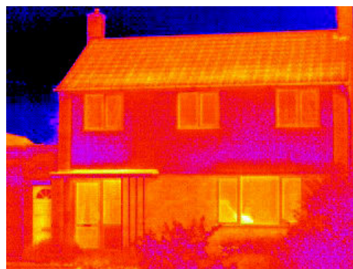
Thermal images clearly showing heat loss
